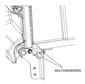
6. Align the rear bumper to hinge brackets and attach with four 8 mm bolts. Two on driver side and two on passenger side. Tighten bolts to the values found in the torque chart.
